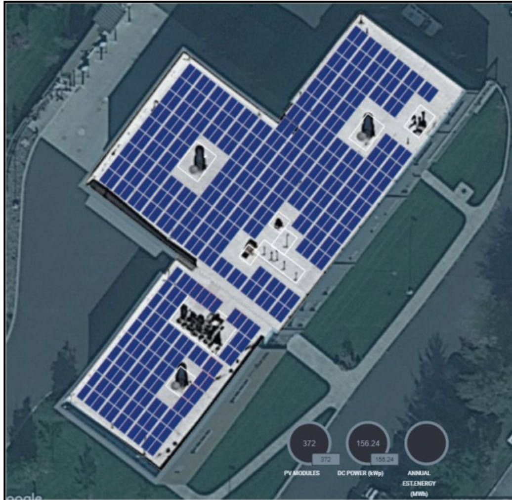
PW Main Building – 156.24 kW DC
